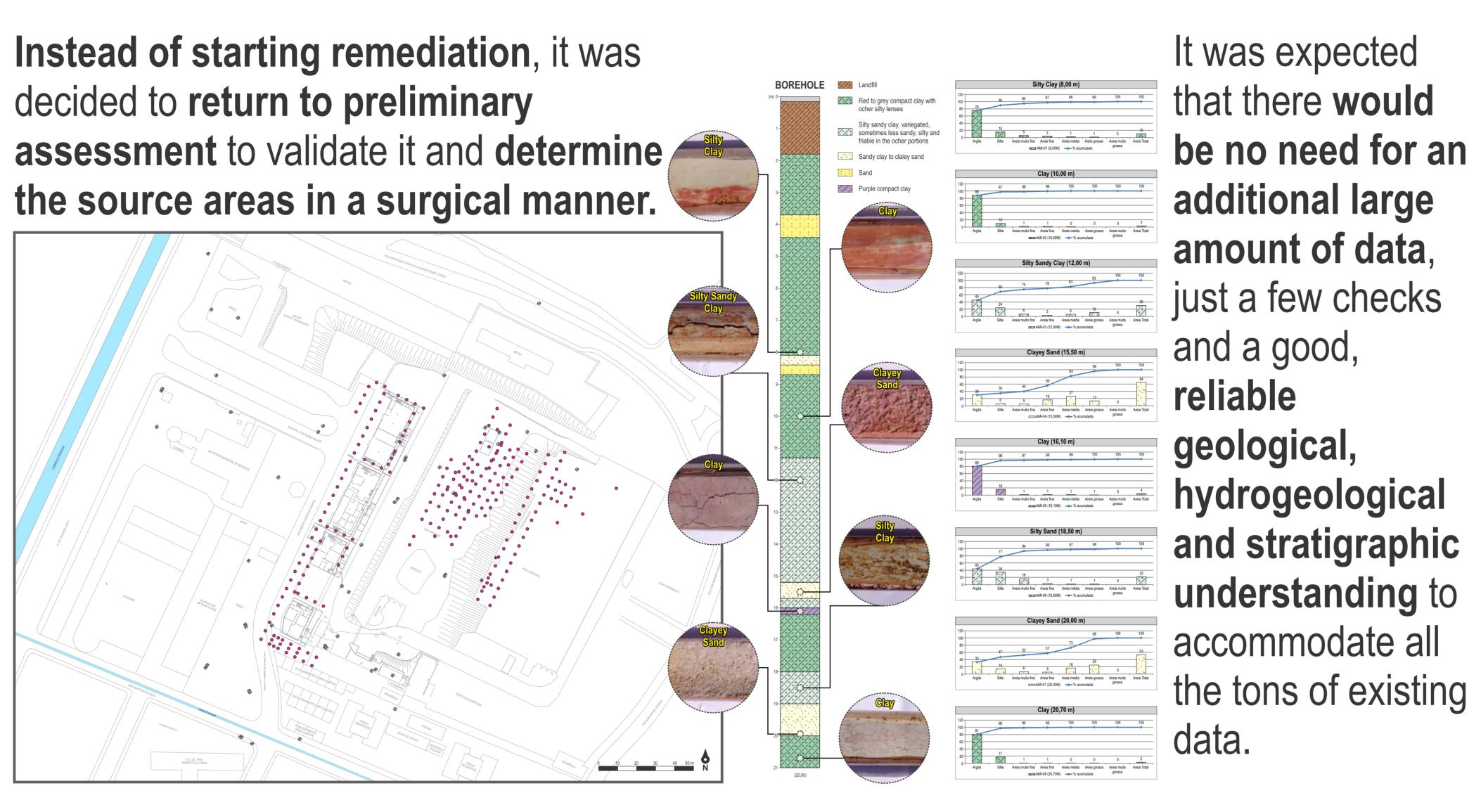
The data were centimetrically correlated to determine an accurate stratigraphic model. Clay levels were compact and thick, providing confinement. Highly permeable horizontal sandy levels (0.5 to 3 meters
